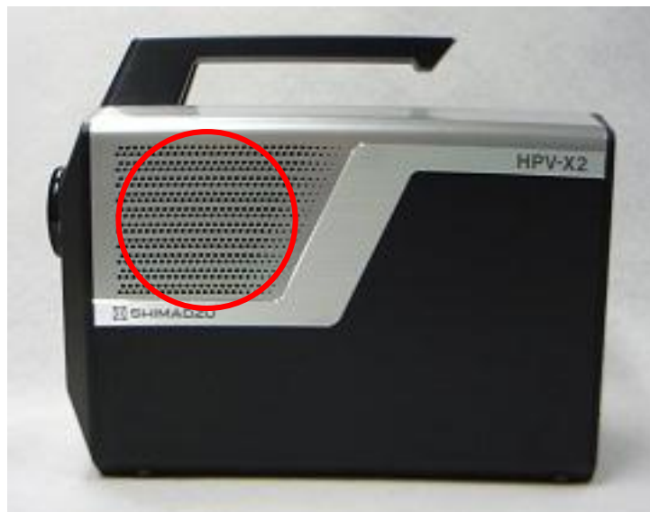
Fig. 6-1 Cleaning the Air Intake Port
