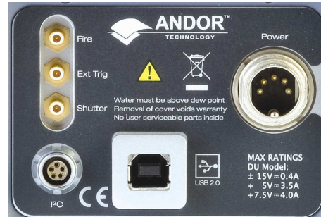
Figure 4: iKon-M rear connectors
