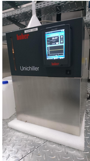
Fig. 3.2: The Huber Unichiller for cooling of the electronics outside vacuum in the wings of AGIPD.
