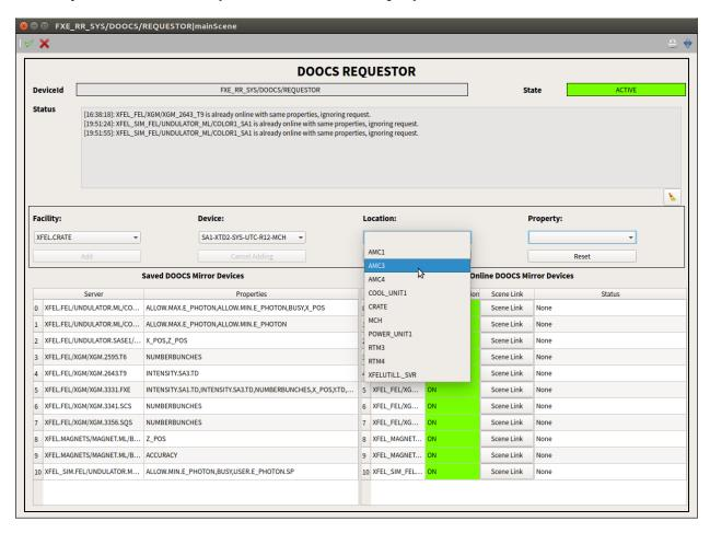
Note that after the selection is made in all of the drop down lists, the device goes to the FILLING state
