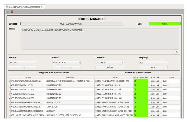
A series of drop-down selections following the DOOCS nomenclature (**Facility**, **Device**, **Location**, **Property**) allows the user to browse across for DOOCS locations and select the DOOCS properties that need to be accessed via Karabo.
