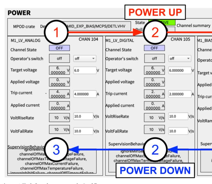
As suggested by the figure, the power-up procedure is as follows:
