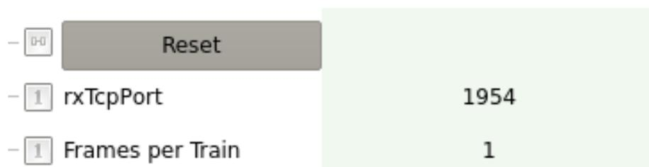
Fig. 2.3: Detail of a JUNGFRAU RECEIVER device, showing the RX TCP Port field
