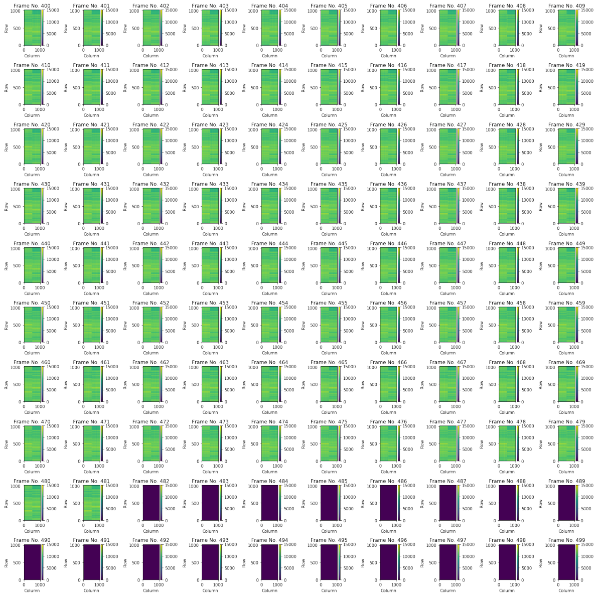
Fig. 2.1: An overview plot showing the last 100 raw (no corrections applied) dark image frames of run number 1 from proposal 2714. In this case the last 18 image frames are empty because the total number of frames in this run were 482 instead of 500. These 18 empty frames need to be excluded prior to calculating the offset.
