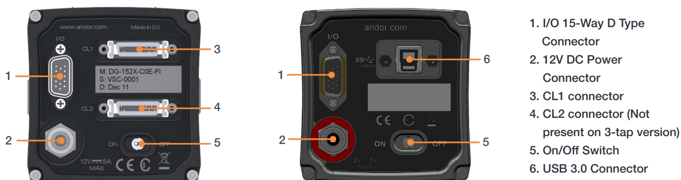
Figure 3: Zyla Back Plate Connections (Left) Cameralink versions (Right) USB 3.0 version
