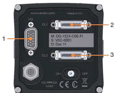
Figure 37: Connect the Zyla to the port on the PC by the connections shown above (Left) Camera Link model, (Right) USB 3.0 model
