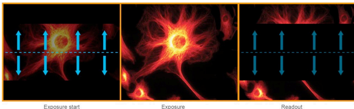
Figure 8: Rolling Shutter Exposure and Readout
